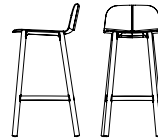
Bar Stool 450mm x 480mm x 940mm H (750mm seat height) 450mm x 480mm x 840mm H (650mm seat height)
